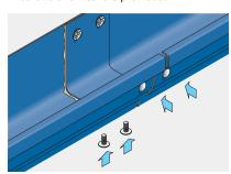
Slide in union joint and insert gutter bolts (heads outside). Secure joint with nuts and washers taking care not over tighten or displace sealant from within the joint.
