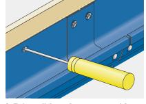
Tighten all fascia fixing screws and fit top straps if required otherwise screw back securely to the fascia using No12 x 38mm round head wood screws and washers provided.
