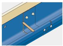
Tool off excess silicone and cone-off the exposed washers and nuts inside the gutter with a generous application of silicone sealant.
